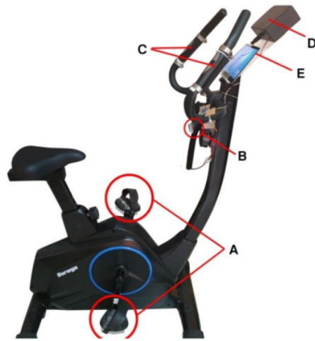
Figure 1. Virtual cycling simulator; A: pedals with balance modules; B: heart rate module; C: steering on-off module; D: control box; E: central processing and display unit.
