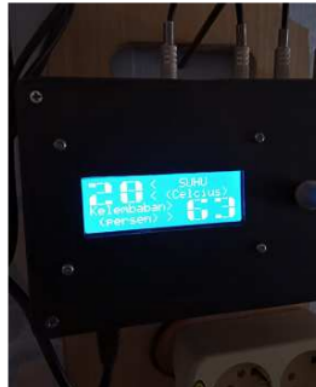
Figure 6.the humidity and temperature showing at DHT-11 sensor
