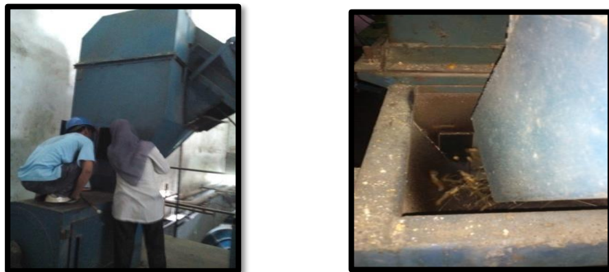
Gambar 4.3 Kegiatan perontokan/pemipilan jagung ( Shelling ) di PT. Asian Hybrid Seed Technologies Indonesia .
