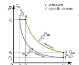
Gambar 1. Diagram P – v Motor Diesel
