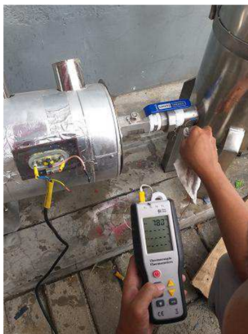
Figure 6.Purification Testing with Temperature 80 0 C
