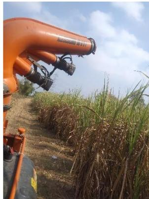
**Gambar 3. 3 Pengoperasian Boom Sprayer**
