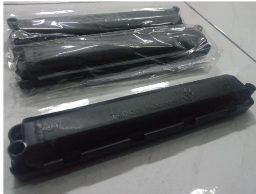
Gambar 3.7 Optical Termination Premise
