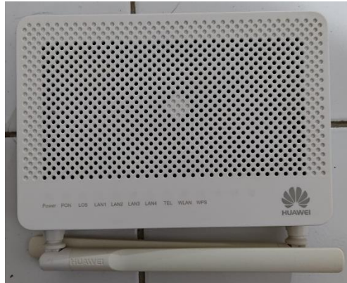
Gambar 4. 6 ONT (Optical Network Terminal)
