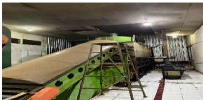
Gambar 3. 25 VFBD (*Vibro Fluid Bad Dryer*)
