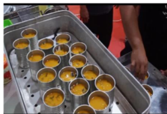
Gambar 2. Proses filling dan exhausting awal ikan lemuru bumbu kuning kaleng
