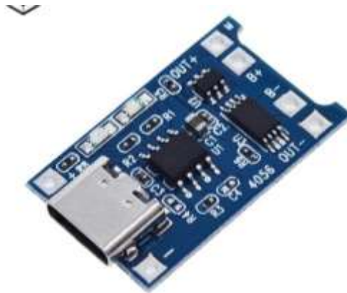
Gambar 2.12 Type-c Power Input
