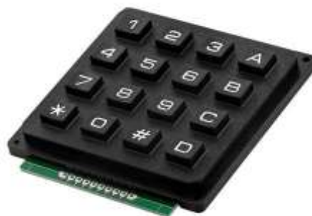
Gambar 2.10 Keypad Matrix 4x4
