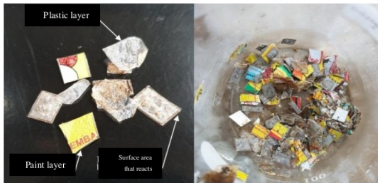
Fig. 9. Samples of used aluminum beverage cans that is not completely reacting
