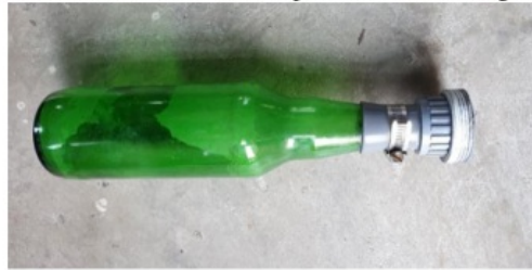
Fig. 5. The hydrogen reactor used glass bottle with a volume of 620 ml
