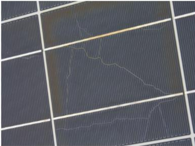
Gambar 4.19 Snail Track (Sumber: ica solar)
