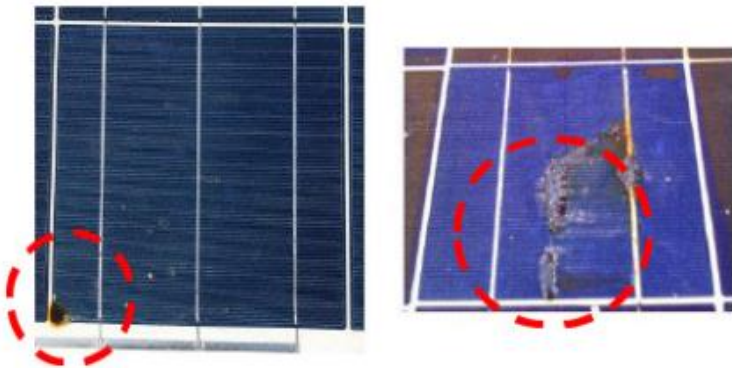
Gambar 5.13 Panel Surya Hotspot (Sumber: USAID)
