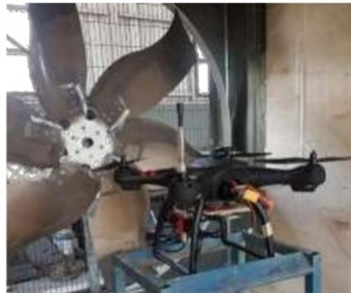
Fig. 6. Complete prototype of anemometer quadcopter surveyor drone.
