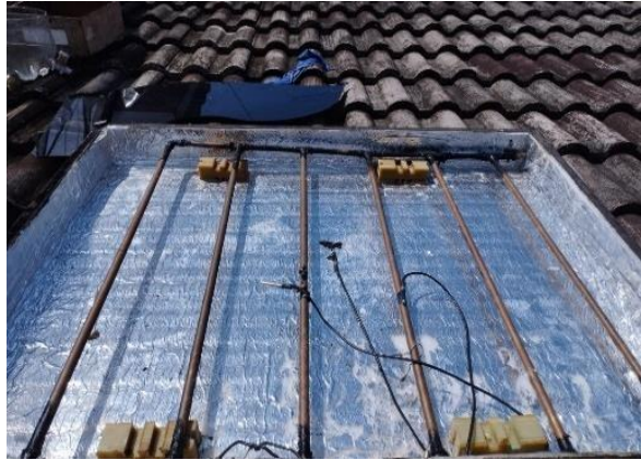
Figure 2. Copper pipe with evaporator chamber.
