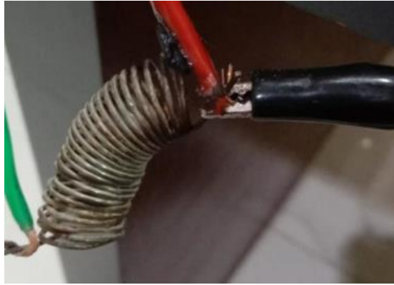
Figure 4. The heater coil mounted on the pipe.
