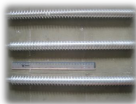
Figure 1. The threads are made with different compression ratio (1.5; 2.5; 3.5)
