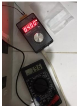
FIGURE 8. Current sensor testing with Generator signal
