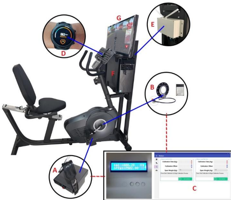
Figure 1. VR system-based cycling components for post-stroke training: (A) pedal module, (B) cadence module, (C) calibration tool and sensors monitoring, (D) heart-rate monitor module, (E) data acquisition box, (F) central processing unit, (G) virtual environment
