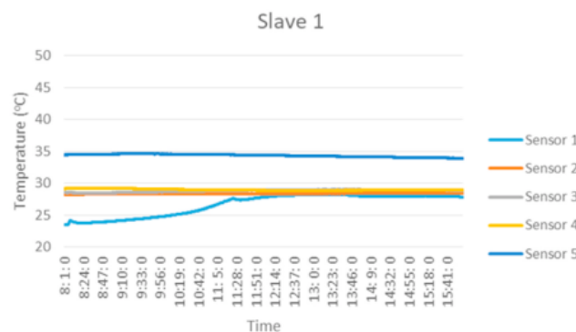
Fig. 5. Temperature measurement graph on slave 1.
