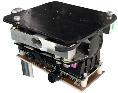
Fig. 3. Pedal design without strap and cover box
