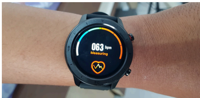
Fig. 5. Wireless physiological parameters monitor: HR, BP, SpO 2
