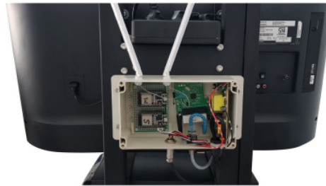
Fig. 6. Data acquisition module behind display screen of virtual environment
