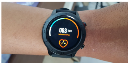
Fig. 5. Wireless physiological parameters monitor: HR, BP, SpO 2
