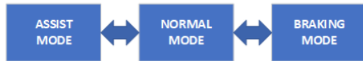
Fig. 4. Switching modes operation to maintain desired cycling cadence to accommodate varying levels in lower extremity impairments
