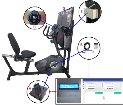
Fig. 1. VR system-based cycling components for post-stroke training; A: pedal module; B: cadence module; C: calibration tool and sensors monitoring; D: heart-rate monitor module; E: data acquisition box; F: central processing unit; G: virtual environment
