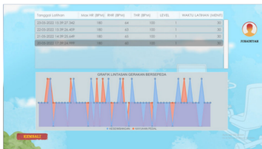
Fig. 9. Logging of the rider's balance and ability to follow the trainer's trajectory at a safe distance
