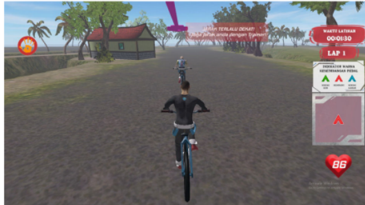
Fig. 8. The virtual environment of the simulator where the rider (behind) follows the cycling track of the virtual trainer (ahead) at a safe distance and monitors heart rate safely during training
