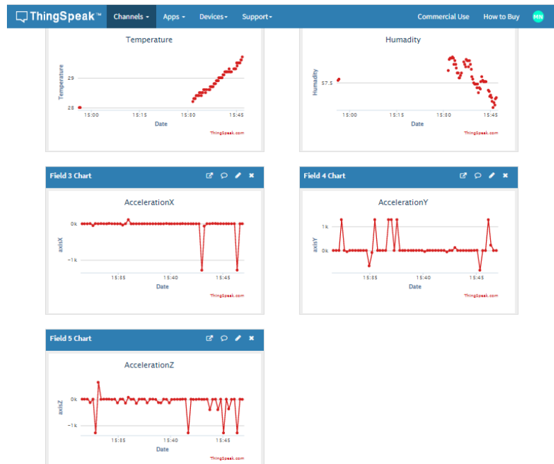
Figure 5. Display on thingspeak.com when gearbox is treated
