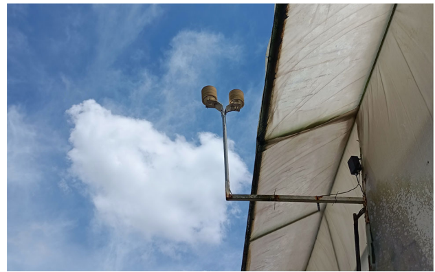
Fig. 19 Humidity and outdoor sensors determine the temperature difference inside and outside the smart green house
