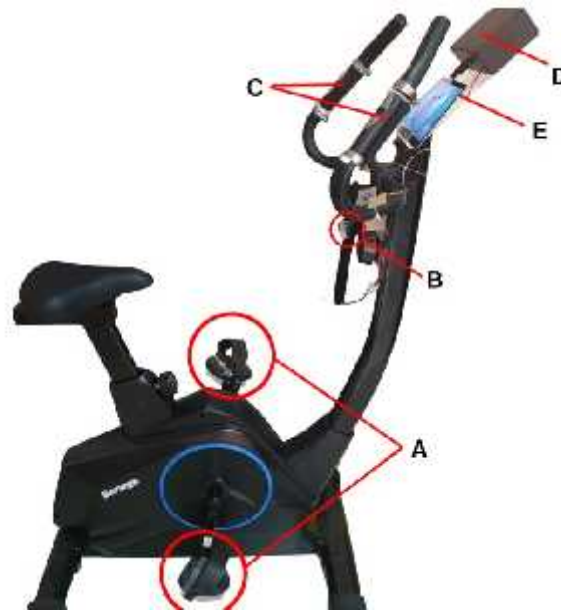
Figure 1. VRAC apparatus; A: pedal module; B: heart rate measurement; C: handlebar module; D: control box; E: VRAC simulator.
