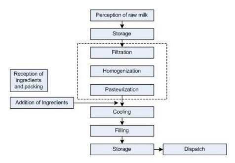
Figure 1. Flow chart of the manufacture of pasteurized fresh milk
