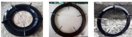
Gambar 1. Perancangan Grid Diameter Lubang 0.4; 0.6; 0.8 cm
