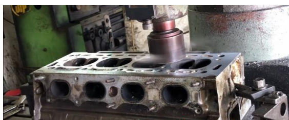
Gambar 4.10 Proses Frais Cylinder Head (Dokumen Pribadi, 2020)
