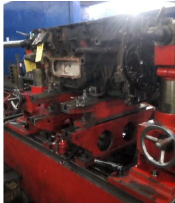
Gambar 4.9 Proses Centering Cylinder Block (Dokumen Pribadi, 2020)
