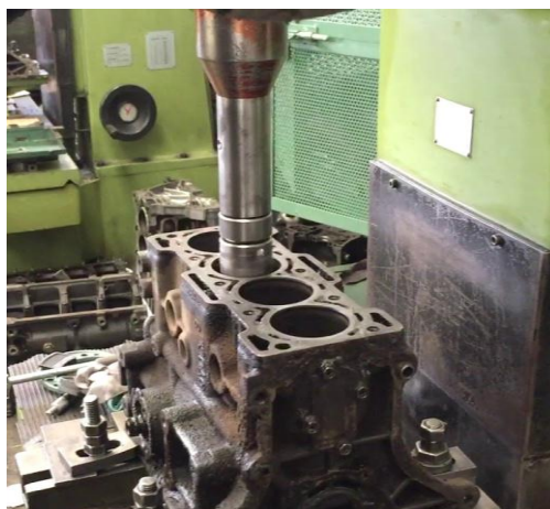
Gambar 4.8 Proses Colter Cylinder Block (Dokumen Pribadi, 2020)
