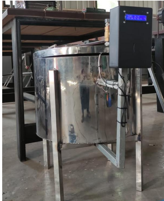
Gambar 5.15 alat Temperature And Fermentation Controlled Chamber (TFCC) dengan Teknologi Hybrid System
