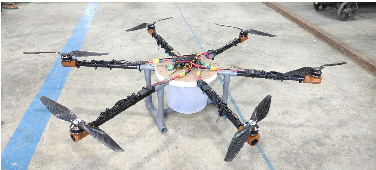
Figure 1. Unmanned aerial vehicle for foliar fertilizer with carbon arm based split tank
