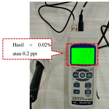
(c) Hasil Pengukuran Kadar Salinitas
