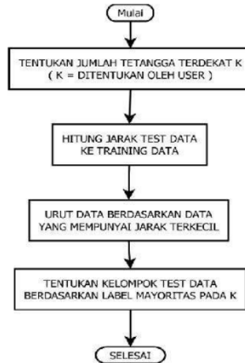
Gambar 3. Flowchart Algorithm KNN
