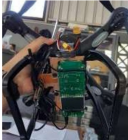
Fig. 3. Integrated anemometer below the drone.
