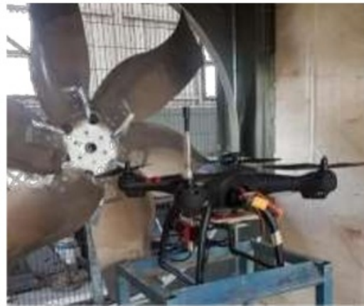
Fig. 6. Complete prototype of anemometer quadcopter surveyor drone.
