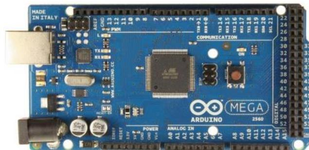
Gambar 2. 2 Arduino Mega
