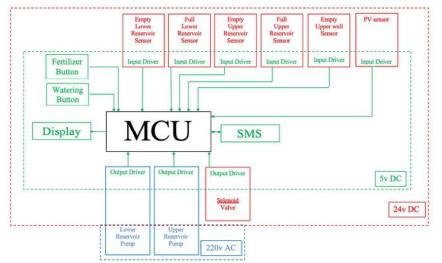
Figure 2. Mobile power and control systems
