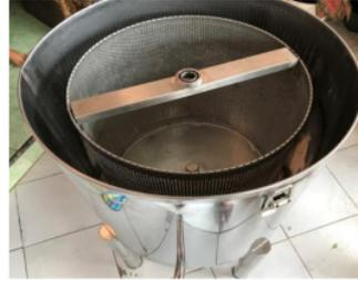
Gambar 3. Desain rancangan tabung putar (*Rotary Drum*)
